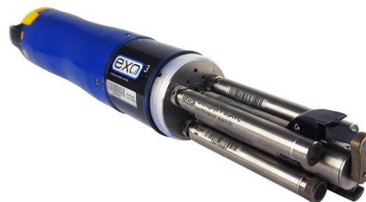
Figure 3.59 The EXO is the YSI instrument used to monitor CWQMN station CAMS749
