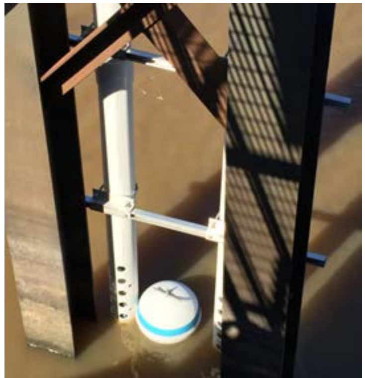
Pictured above are Ed Ragsdale (TCEQ), Joe Parish (LNVA), Chuck Dvorsky (TCEQ), and Zak Sihalla (Hydrotech) who participated in the installation of a newly designed deployment system for the real-time station (CAMS 749) on Pine Island Bayou. Pictured below is the unique deployment system using PVC tubes with a single buoy to float YSI multi-probes located inside each tube for the LDM installation and testing project.
