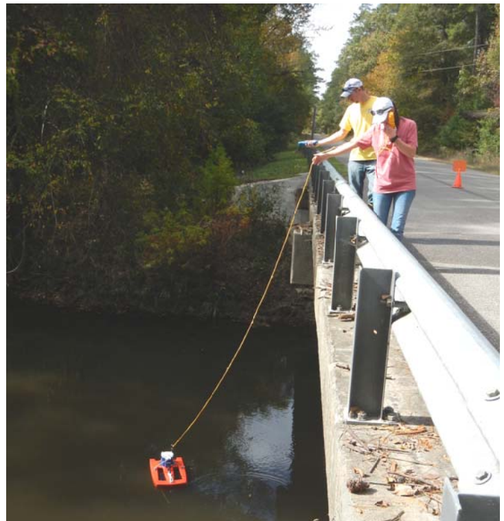
LNVA Environmental Analysts collect stream flow measurements at CRP routine monitoring stations using a Teledyne RD Instruments' StreamPro ADCP (Acoustic Doppler Current Profiler).
